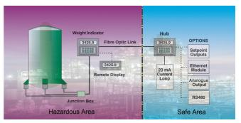
This third example shows a fibre optic link between the hazardous area and the safe area. Full functionality of the ATEX certified Weight Indicator is available through the Hub Terminal in the safe area and an extensive range of communication options complete this flexible and versatile installation. Power to the instrumentation in the hazardous area may come from certified batteries or mains supplies.
