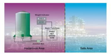
In this example, the complete weighing system is situated in the hazardous area with no link back to the safe area. Power is usually provided from appropriately certified battery packs or mains. Typical applications can range from simple vessel storage systems to bag filling stations.
