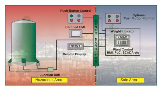
In this conventional hazardous area weighing application, the system integrity is maintained via Zener Barriers. Optional ATEX certified equipment such as remote weight displays or HMIs can be located in the hazardous area, powered from the safe area via the Zener Barriers. Control functions can be carried out in either the safe or hazardous area.
