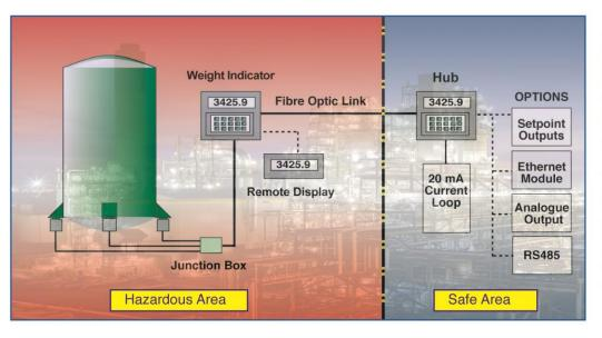
This third example shows a fibre optic link between the hazardous area and the safe area. Full functionality of the ATEX certified Weight Indicator available through the Hub Terminal in the safe area and an extensive range of control and communication options complete this flexible and versatile installation. Power to the instrumentation in the hazardous area may come from certified batteries or mains supplies.
